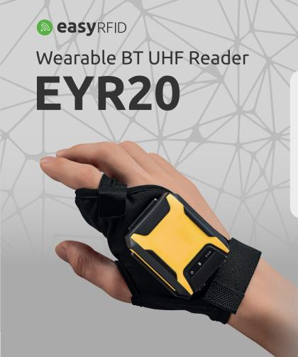
EYR20 is our refined and new generation wearable Bluetooth UHF readers. Being a compact and portable device, it becomes a flexible and practical reading device if attached to gloves, wristbands, or lanyards.
